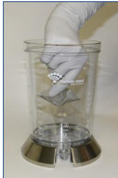
Fig. 3.8: Remove the mesh filter
