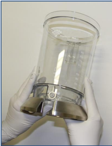
Fig. 3.6: Remove the collection container from the foot ring
