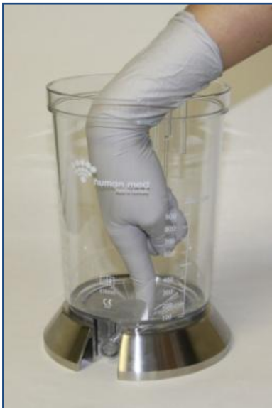
Fig. 3.7: Remove the mesh filter
