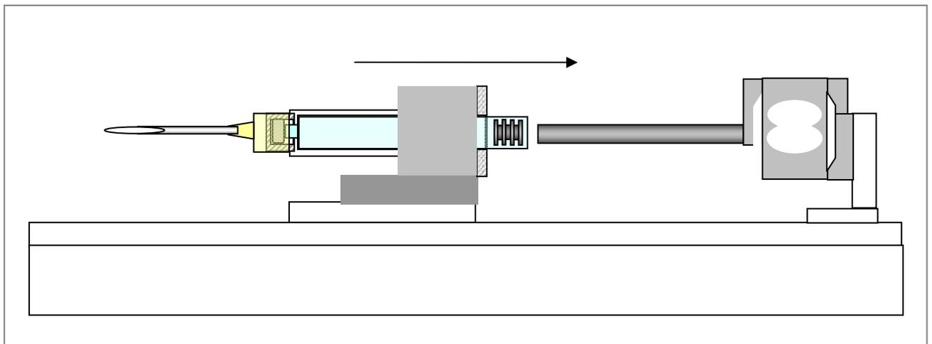
**Figure 4-2: Testing Arrangement of plunger force tests (Application Forces, ISO 11608)**
