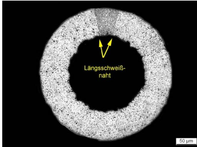
Figure 5-10: KLINON\_29G - Overview, etched, longitudinal weld
