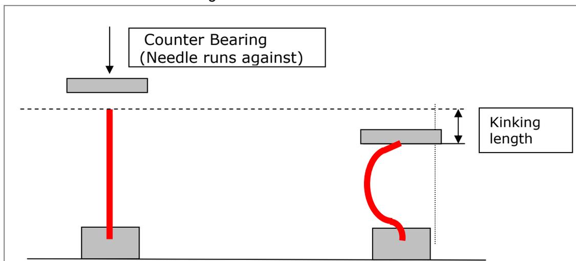
Figure 4-3: Arrangement of the kinking test
