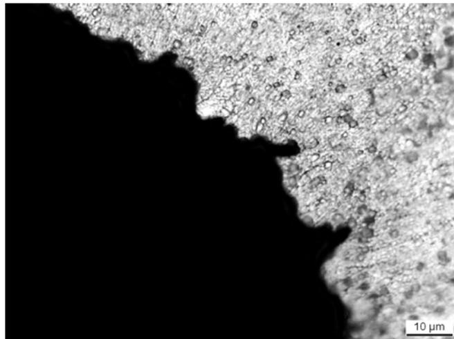
Figure 5-11: KLINON\_29G – Internal surface, wide die marks up to 12 µm depth
