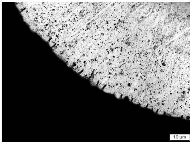
Figure 5-21: BD\_31G - Outer surface, die marks up to 7 µm depth
