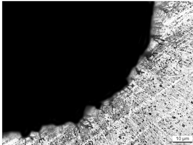
Figure 5-20: BD\_31G - Internal surface, folds up to 8 µm depth
