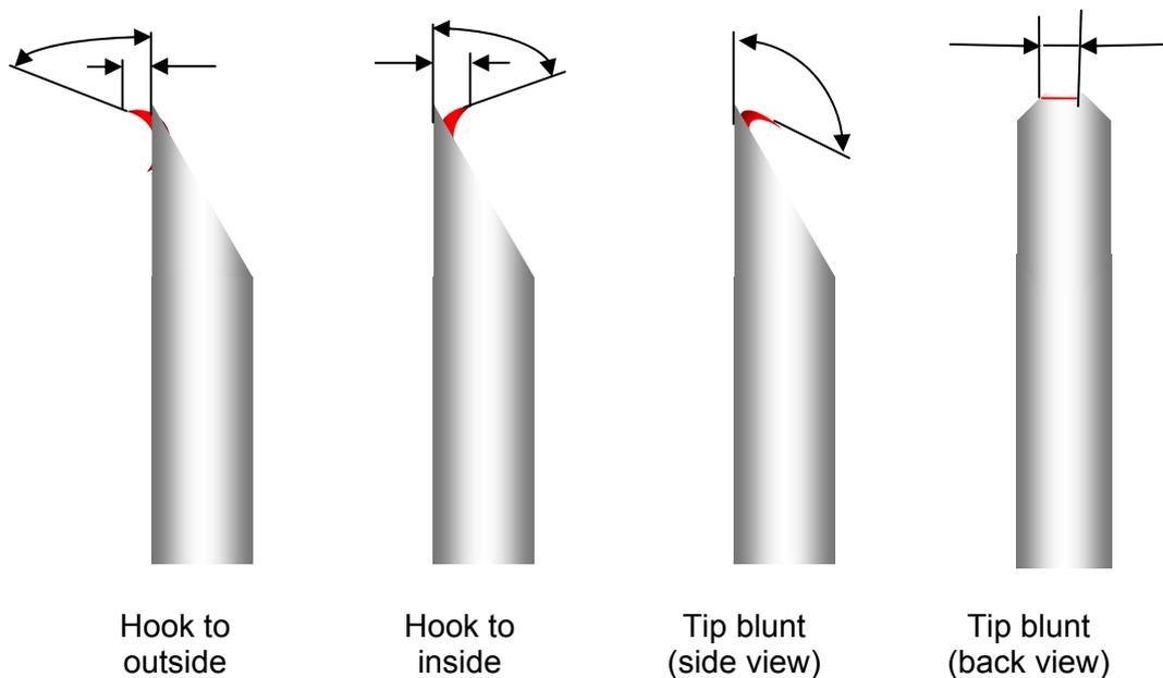
**Figure 5-1: Tip defects**
