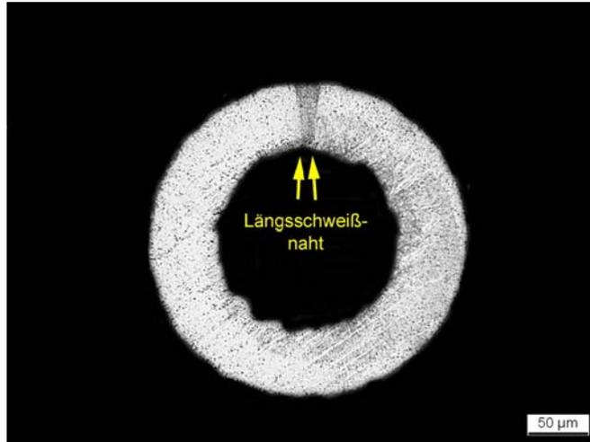
Figure 5-19: BD\_31G - Overview, etched, longitudinal weld
