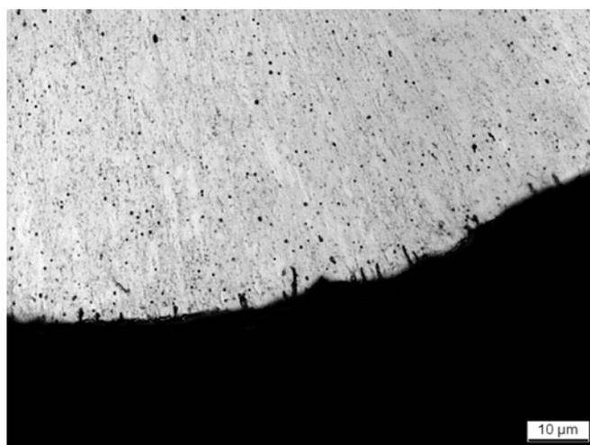
Figure 5-15: BD\_29G – Outer surface, die marks up to 5 µm depth
