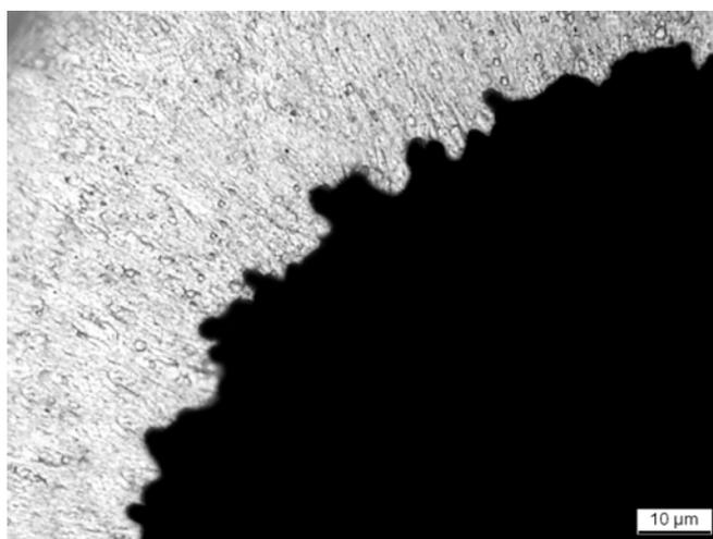
Figure 5-17: KLINON\_31G - Internal surface, wide die marks up to 7 µm depth
