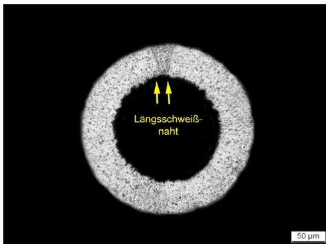
Figure 5-16: KLINON\_31G - Overview, etched, longitudinal weld
